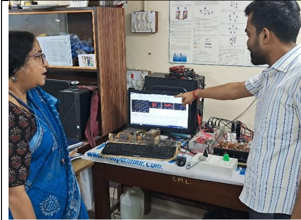
PR Controlled Single Phase Inverter using d-Space 1104
