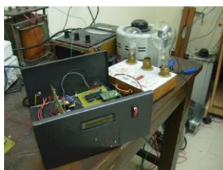
Fig. 14 Testing of EM Assembly with R-L Load
