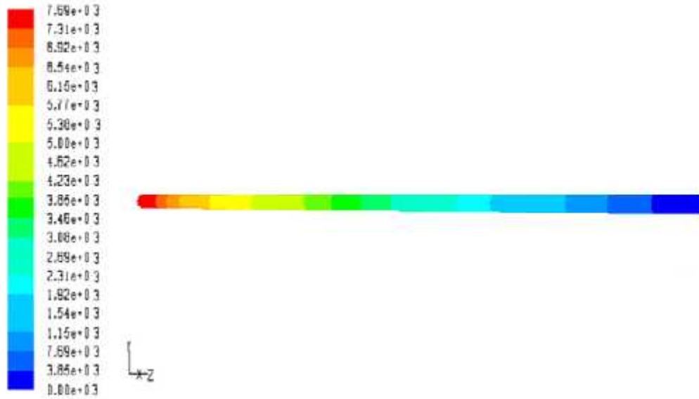
Fig. 5.2 Contour plot of static pressure for straight pipe Concentration of SMC solution ( \text{kg/m}^3 ): 0.8, Liquid velocity (m/s): 0.3199
