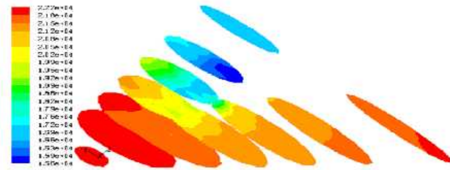
Fig. 5.11a Contours plot of static pressure inside the different points of 45 0 elbow Concentration of SMC solution (kg/m 3 ): 0.8, Liquid flow rate, Q 1 (m 3 /s): 21.94x10 -5 , Liquid velocity, V 1 (m/s): 1.733
